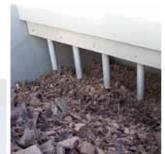
In 2002 Saxlund International Ltd supplied a tyre chip truck reception bunker equipped with the Saxlund Push Floor discharge machine at the existing Ribblesdale Tyre Chip Handling Plant. The Push Floor discharges the tyre chips to our metering belt conveyor with scalping drum and belt weighing system. This conveys the material in a metered fashion from the bunker to the Bucket Elevator.
